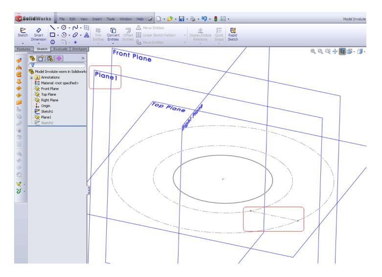
3. On the new sketch plane draw a line at lead angle on the base diameter.You can calculate the lead angle on the base diameter from:Angle = atn(lead/Pi/base diameter)
