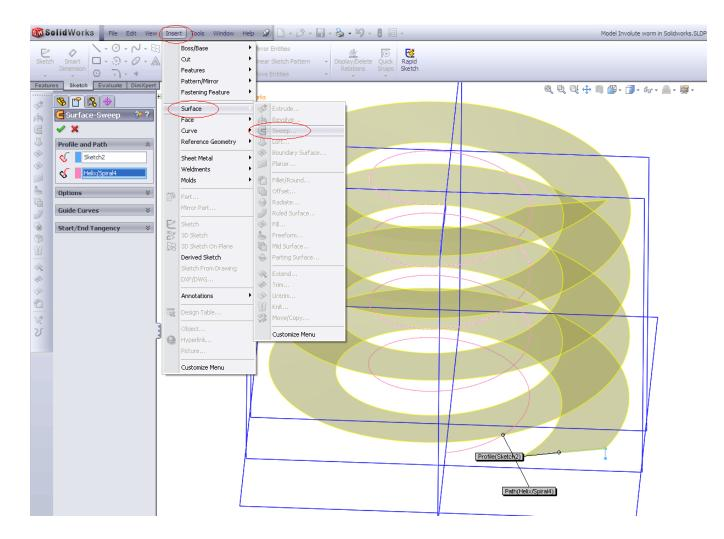
Note, that this is a theoretical surface. This method is using the property of the involute helical surface – it is form by a straight line moving along a helix – like helical winding a string on a tube. However, the real production worm will have a protuberance on the root generated by the manufacturing tool. Contact spiralbevel.com to get software for accurate 3d CAD modeling of the realistic production worm.
